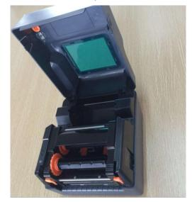
3. Make the left side of recovery shaft (Hexagonal side) pressed into the ribbon recovery wheel,
