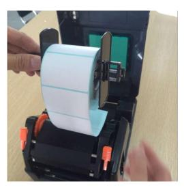
4. Press the printing head switch to open the printing head
